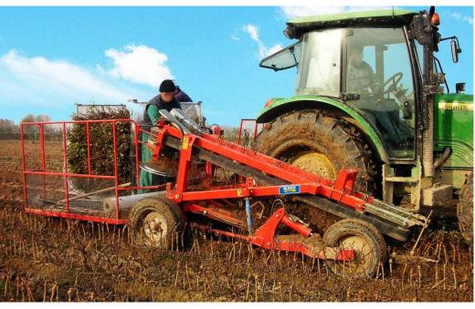
The Harvester machine SP2000 is a machine conceived for: harvesting and digging out of rootstocks, vine cuttings; cleaning their roots from soil; sorting and storage of nursery plants
