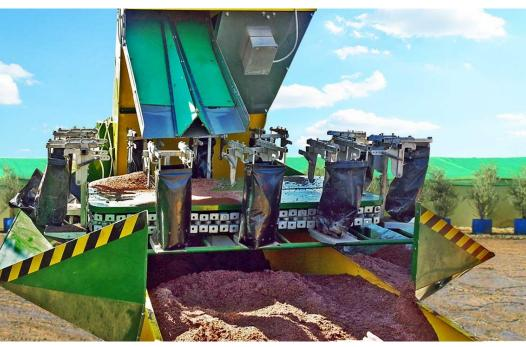
The Soilbagger machine is perfect for the **nylon soil bags for nurseries packaging** for large productions. Suitable for **bagging soil**, **compost**, **humus**, **peat and various substrates**.
