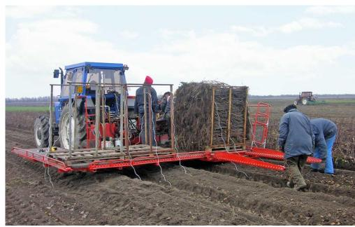
The SP96 Harvesting Machine is a machine designed for: excavation, collection, sorting, storage of nursery plants, on any type of soil, particularly hard / heavy / clayey.
